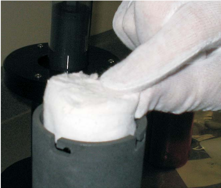
Figure 16 Place insulation in cell basket
