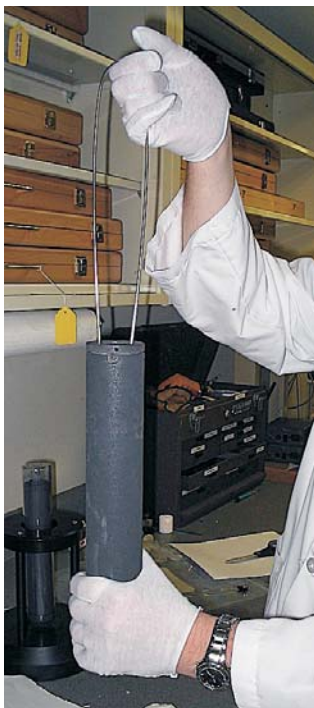
Figure 24 Preparing basket assembly for installation in furnace.
