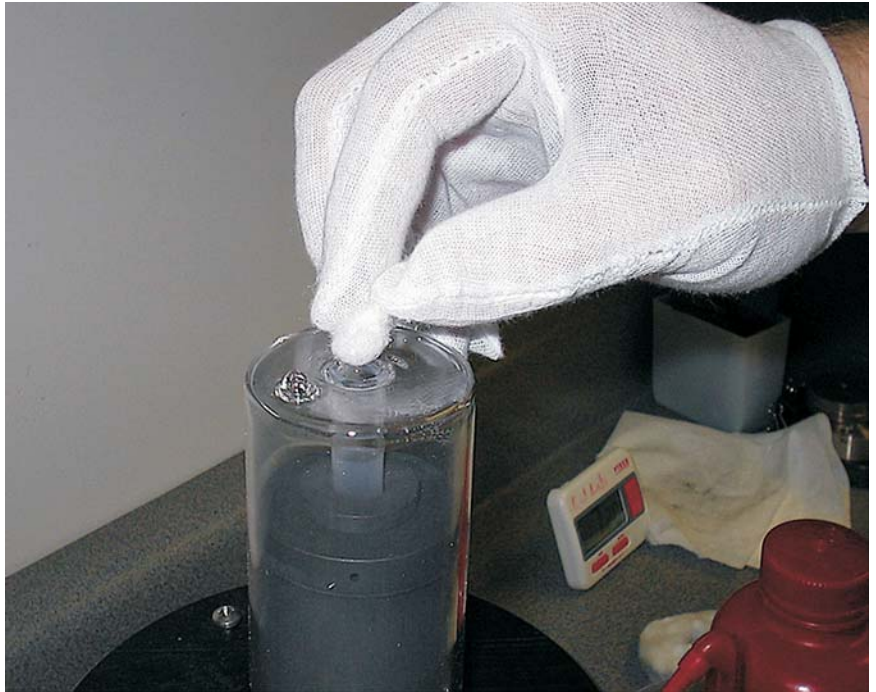
Figure 13 Place insulation in re-entrant well.
