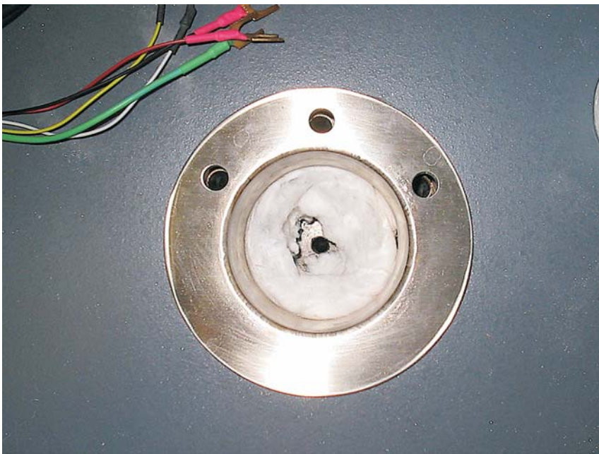
Figure 27 Basket, insulation, and furnace lid installed .
