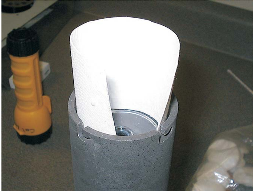
Figure 21 Place fiber ceramic paper to center the cell in cell basket.
