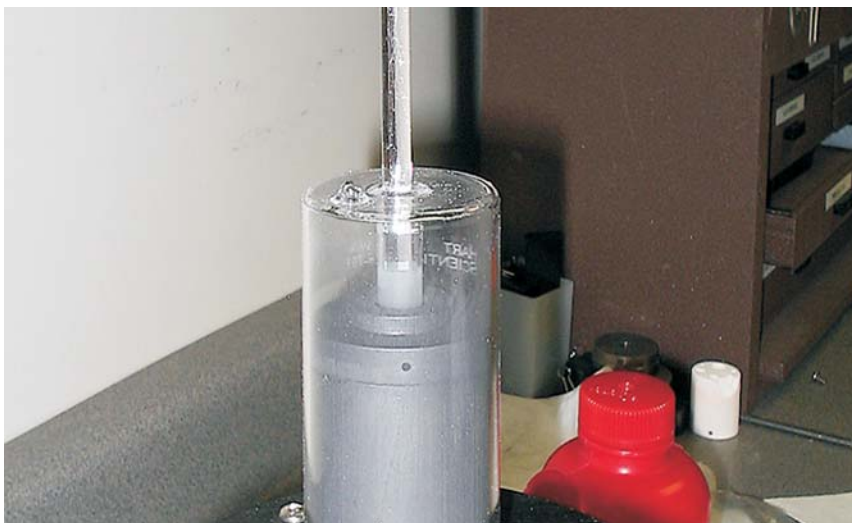
Figure 14 Push insulation to bottom of re-entrant well.
