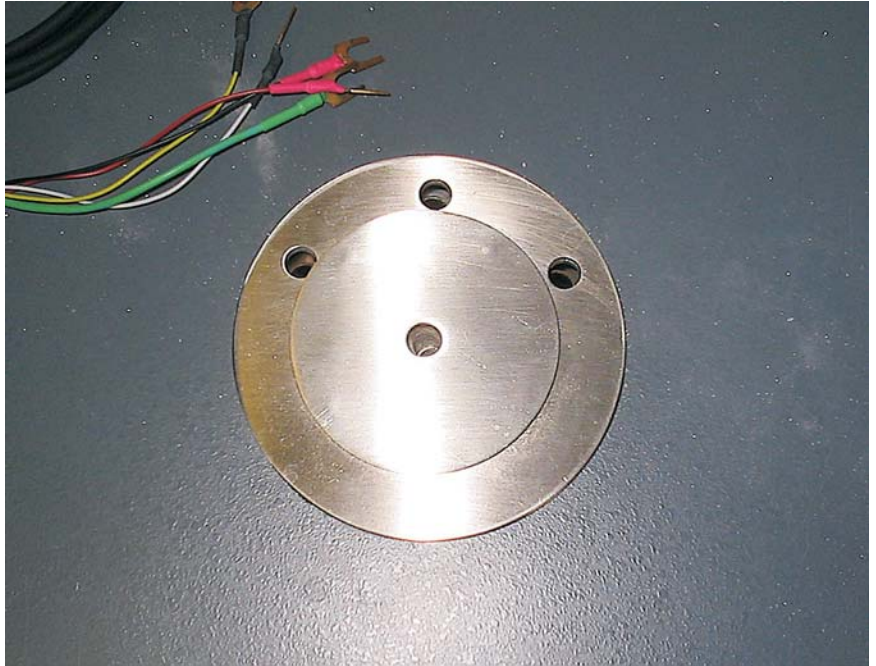
Figure 28 Heat radiation guard installed.
