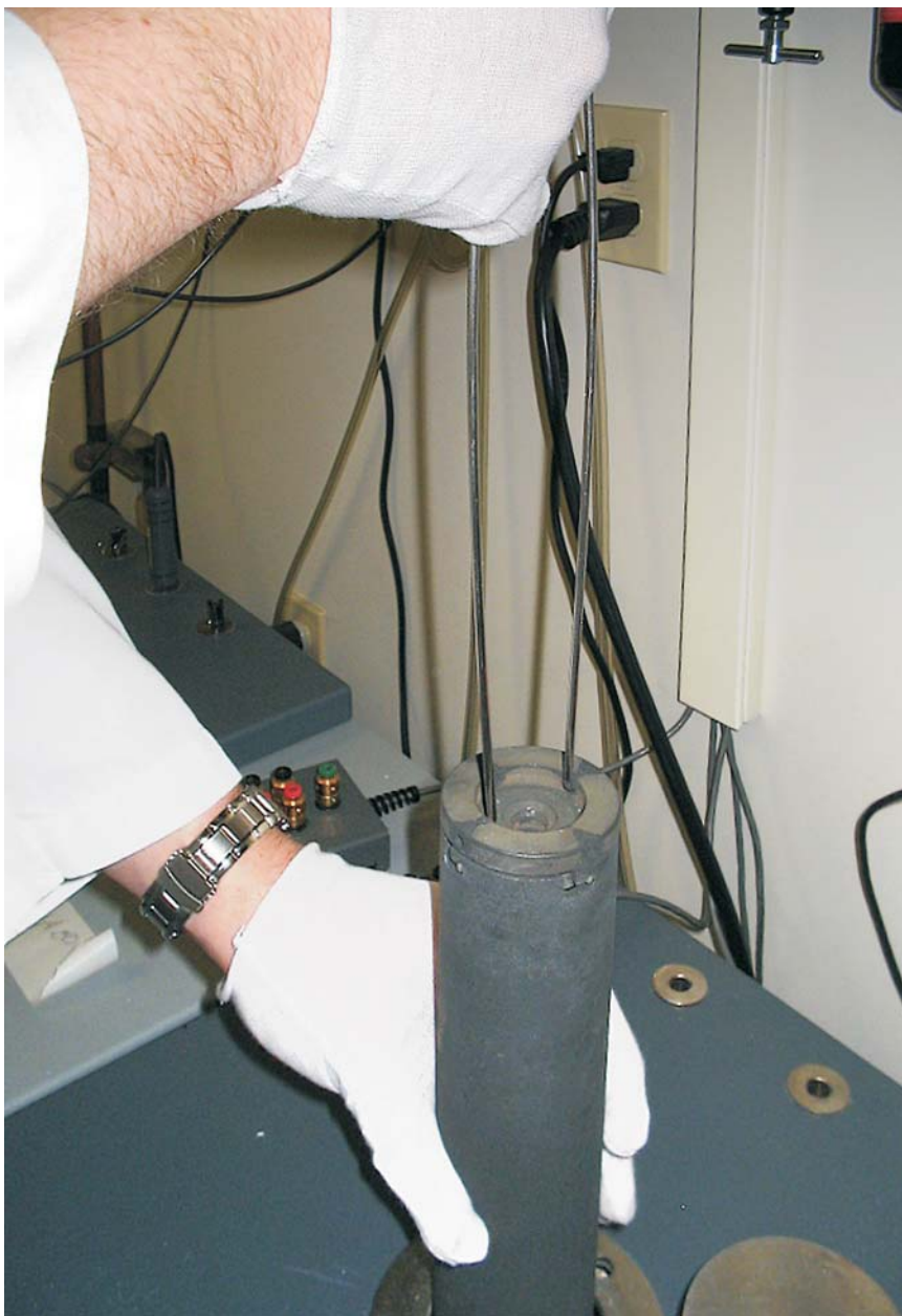
Figure 25 Installing basket assembly in furnace.
