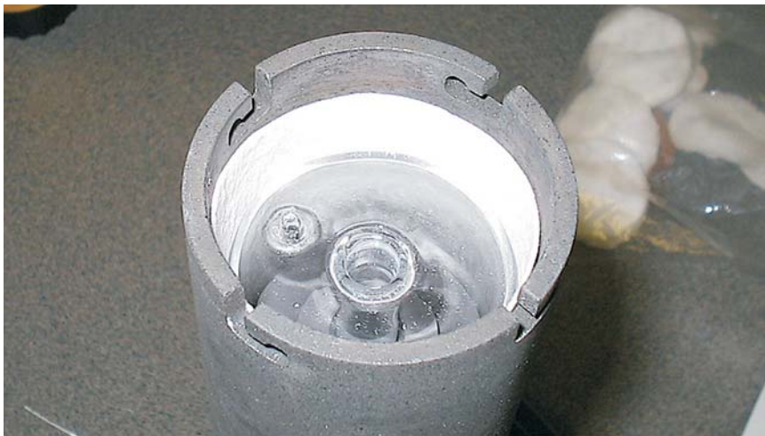
Figure 23 Fiber ceramic paper pushed below cell basket top.
