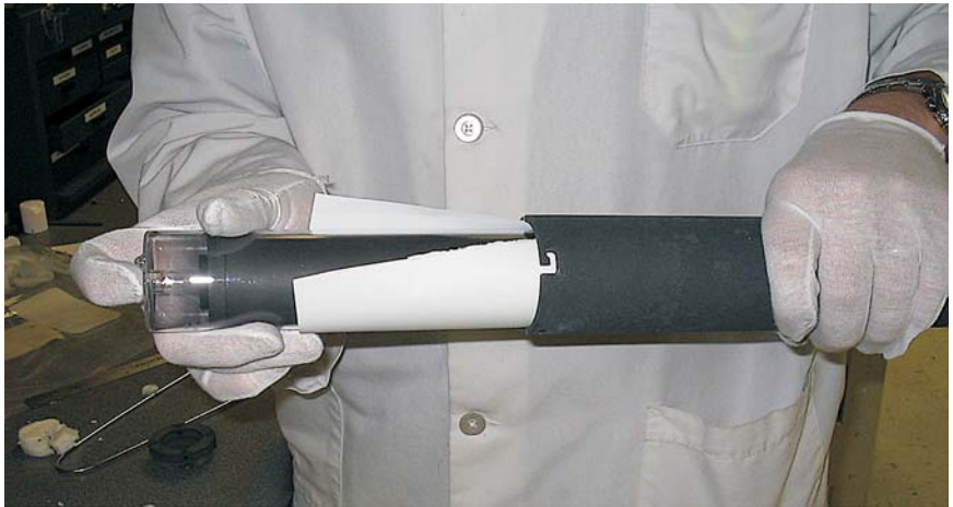
Figure 20 Insert cell into basket.
