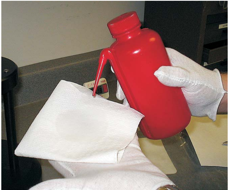
Figure 11 Preparing paper towel with reagent grade alcohol.
