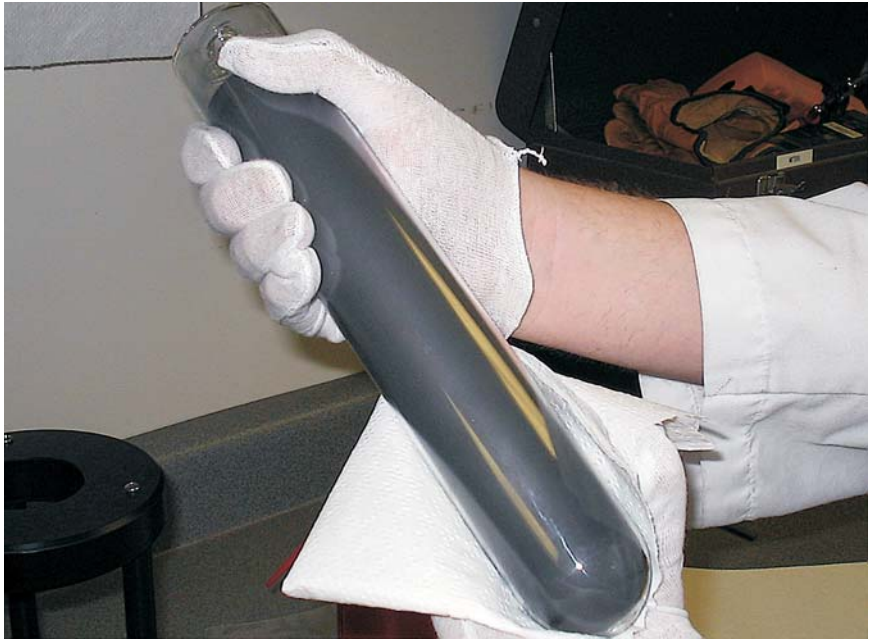
Figure 12 Clean cell completely.
