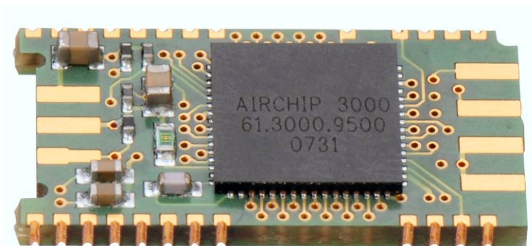
AirChip 3000 installed on its small companion PCB
